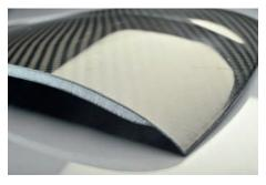
Image: ROHACELL<sup>®</sup> foam forms the core of lightweight sandwich structures with high shear strength and compressive strength, even at relatively high temperatures. (© Evonik)
