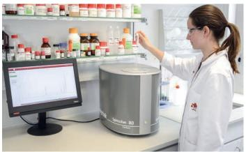
conditions for solvent suppression methods to work. The ULTRA models are ideal to quantify sub-millimolar concentrations of substances dissolved in neat protonated solvents. Besides saturating the signals of the solvent, which can be more than 10.000 larger that the signals of interest, the suppression method offered with the Spinsolve also includes carbon decoupling to eliminate the signal of the carbon satellites of the main solvent signals.
