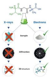
Conventional methods (X-ray) fail because they require big crystal sizes, which are often difficult or even impossible to produce. An electron diffractometer for 3D-structural analysis can deal with nano-crystalline compounds.
