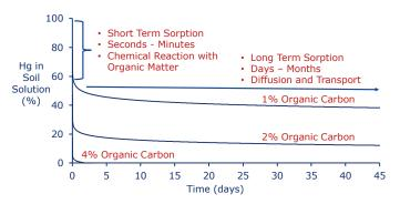
Temporal reduction in the solution phase concentration of Hg added to soil microcosms. The sorption kinetics of Hg were modelled using a parameterized Elovich expression fitted to the experimental data of <sup>196</sup>Hg<sup>+2</sup> sorption in soils with different properties. Modelled lines are displayed for a range of soil organic carbon values at a fixed pH of 4.4.
