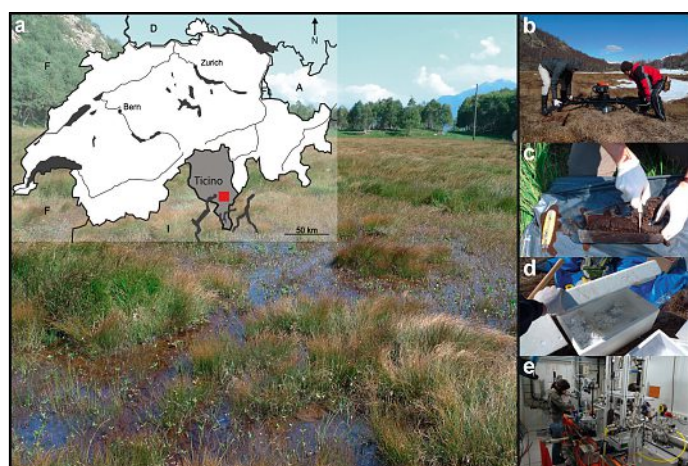
Fig. 1. The field site Gola di Lago (red square) is situated in canton Ticino, Switzerland (a). In order to preserve the element speciation in the samples, retrieved peat cores were rapidly cut into slices, shock-frozen, and stored on dry ice for transportation to the laboratory (b–d). After anoxic sample preparation, selected samples were measured at beamline BM29 of the European Synchrotron Radiation Facility (ESRF, Grenoble, France) (e).
